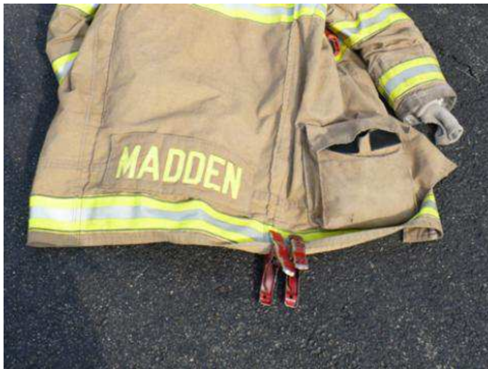
Sgt. Scott Madden from Loudoun County (VA) sent in an idea he got from one of his brothers at Station 6. The idea is to use a small spring hand clamp to wedge doors open. Scott points out that the clamps work well in a number of different ways, and on various types of doors. The photos below show a few of the many options.
