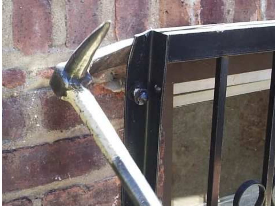
At least one side of the window is not set-up perfectly for using the pike as leverage.
